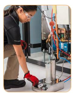
Trained service technicians perform the tests using a documented procedure based on HTM0101 and EN285 standards. The series of tests is performed three (3) times in order to verify repeatable results.
